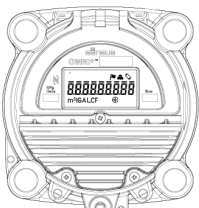
Segment Test View
